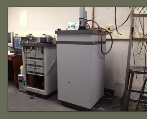
Utilizes temperatures as 2 K and varying magnetic fields to apply a voltage or current to test a materials response
