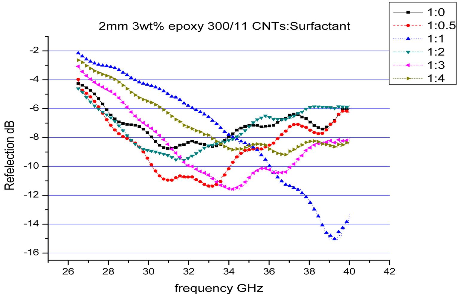
Figure 7 shows that the composites with different ratios of MWCNT/SDBS have different reflection loss properties.
