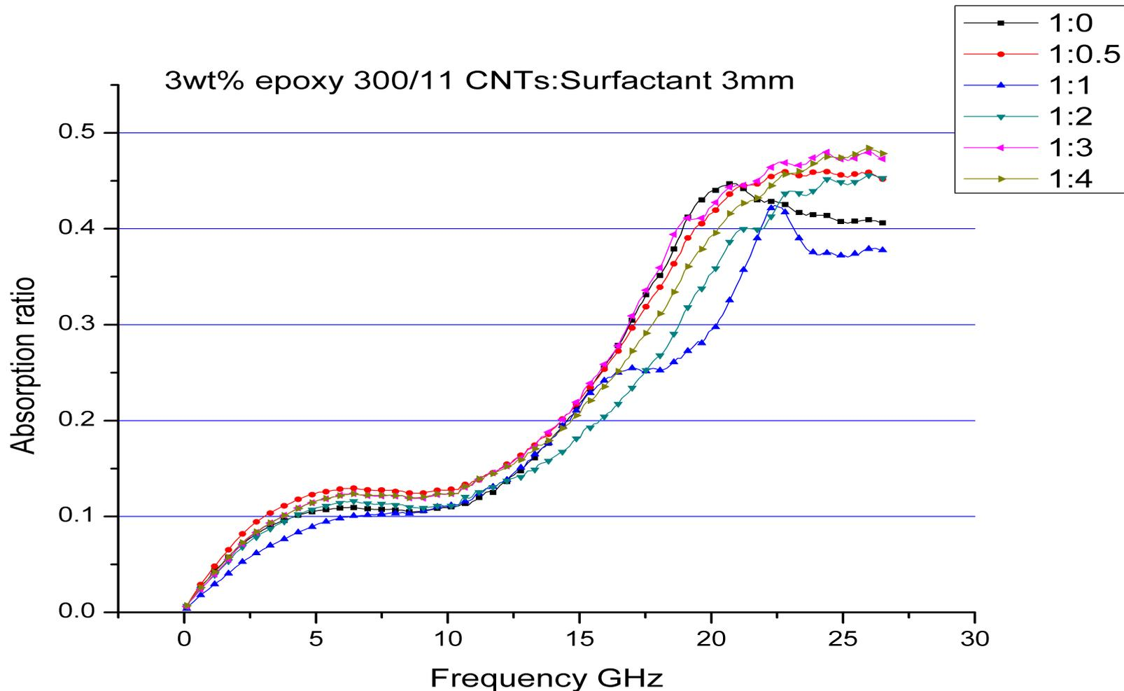
Figure 5 shows that the composites with different ratios of MWCNT/SDBS have different absorption ratios.
