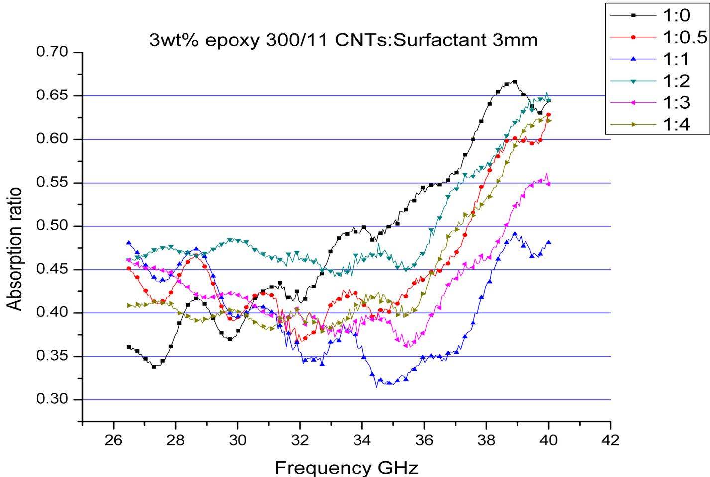
Figure 11 shows that the composites with different ratios of MWCNT/SDBS have different absorption ratios.
