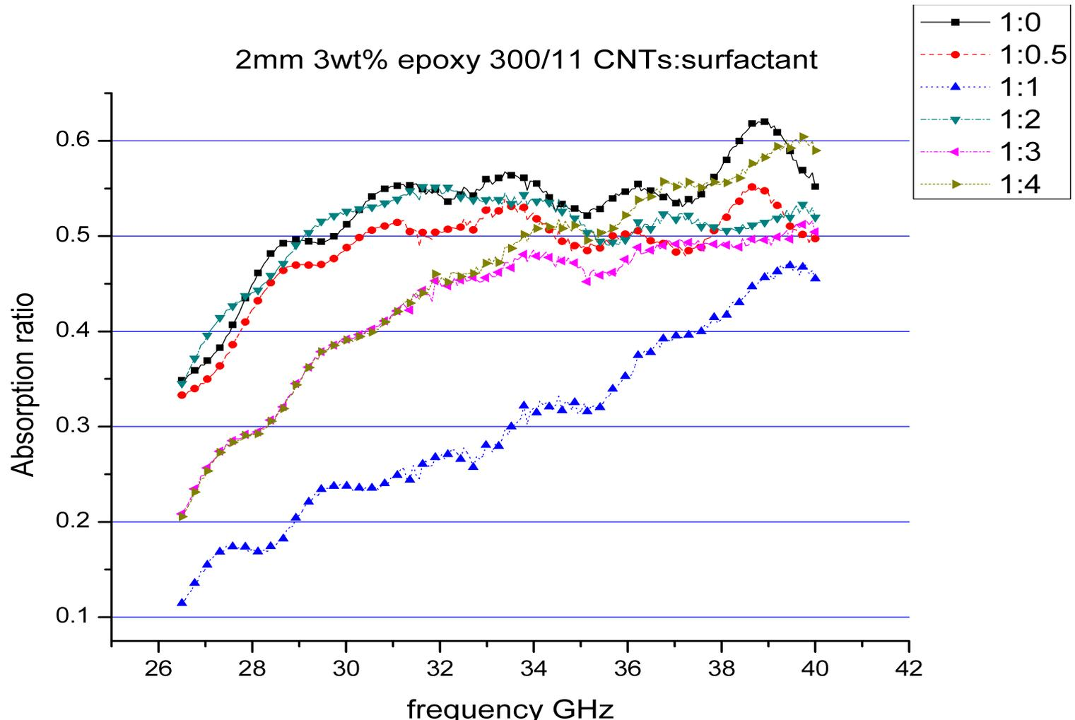
Figures 12 shows that the composites with different ratios of MWCNT/SDBS have different absorption ratios.
