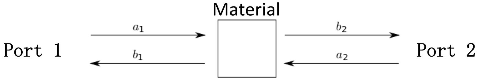
$$S_{11} = \frac{b_1}{a_1}, S_{21} = \frac{b_2}{a_1}, S_{12} = \frac{b_1}{a_2} \text{ and } S_{22} = \frac{b_2}{a_2}$$
