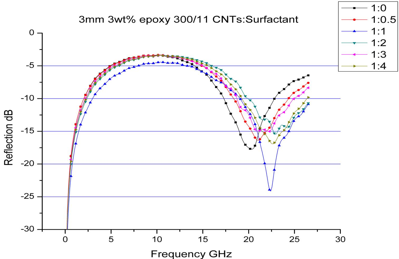
Figures 1 shows that the composites with different ratios of MWCNT/SDBS have different reflection loss properties.
