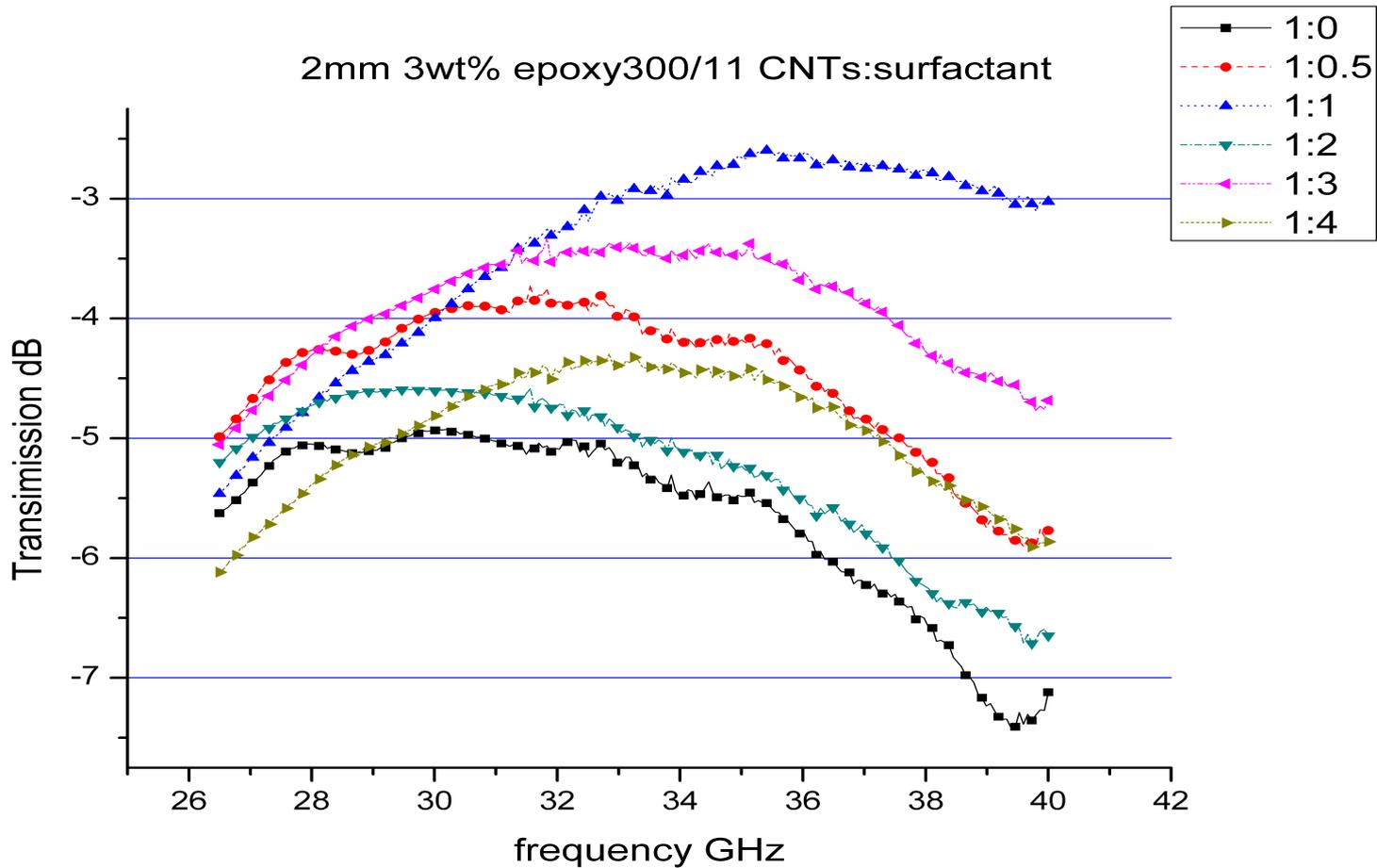
Figure 10 shows that the composites with different ratios of MWCNT/SDBS have different transmission loss properties.
