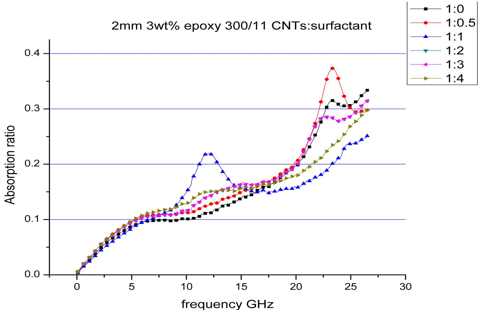
Figure 6 shows that the composites with different ratios of MWCNT/SDBS have different absorption ratios.
