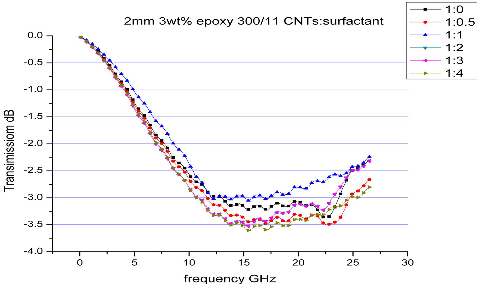
Figure 4 shows that the composites with different ratios of MWCNT/SDBS have different transmission loss properties.
