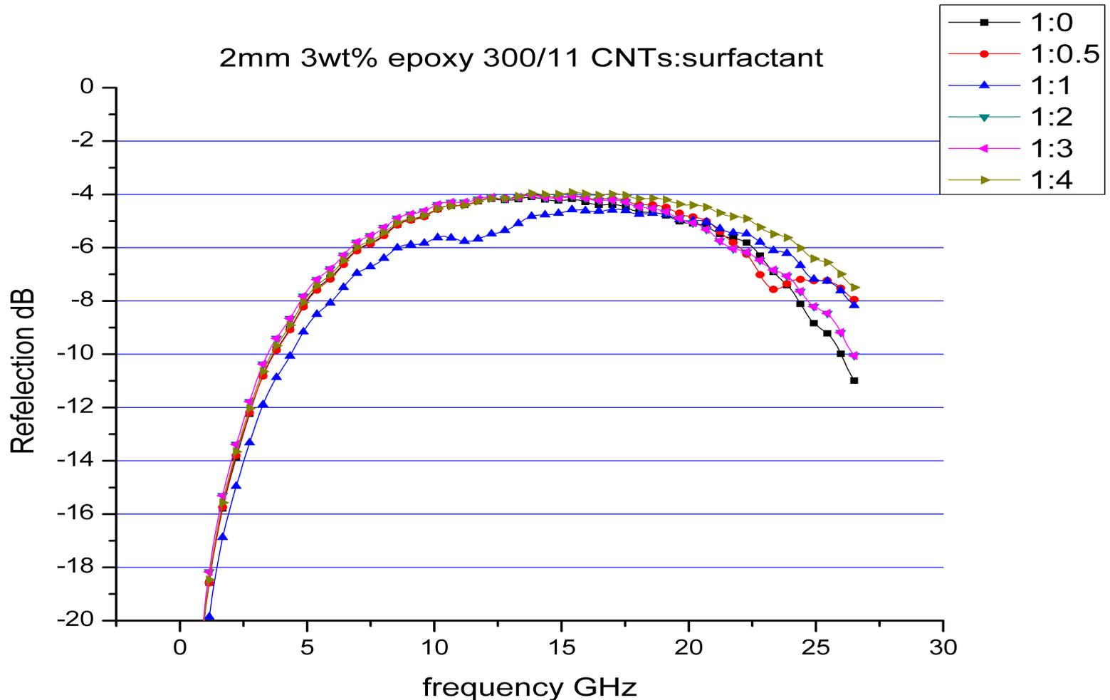
Figure 2 shows that the composites with different ratios of MWCNT/SDBS have different reflection loss properties
