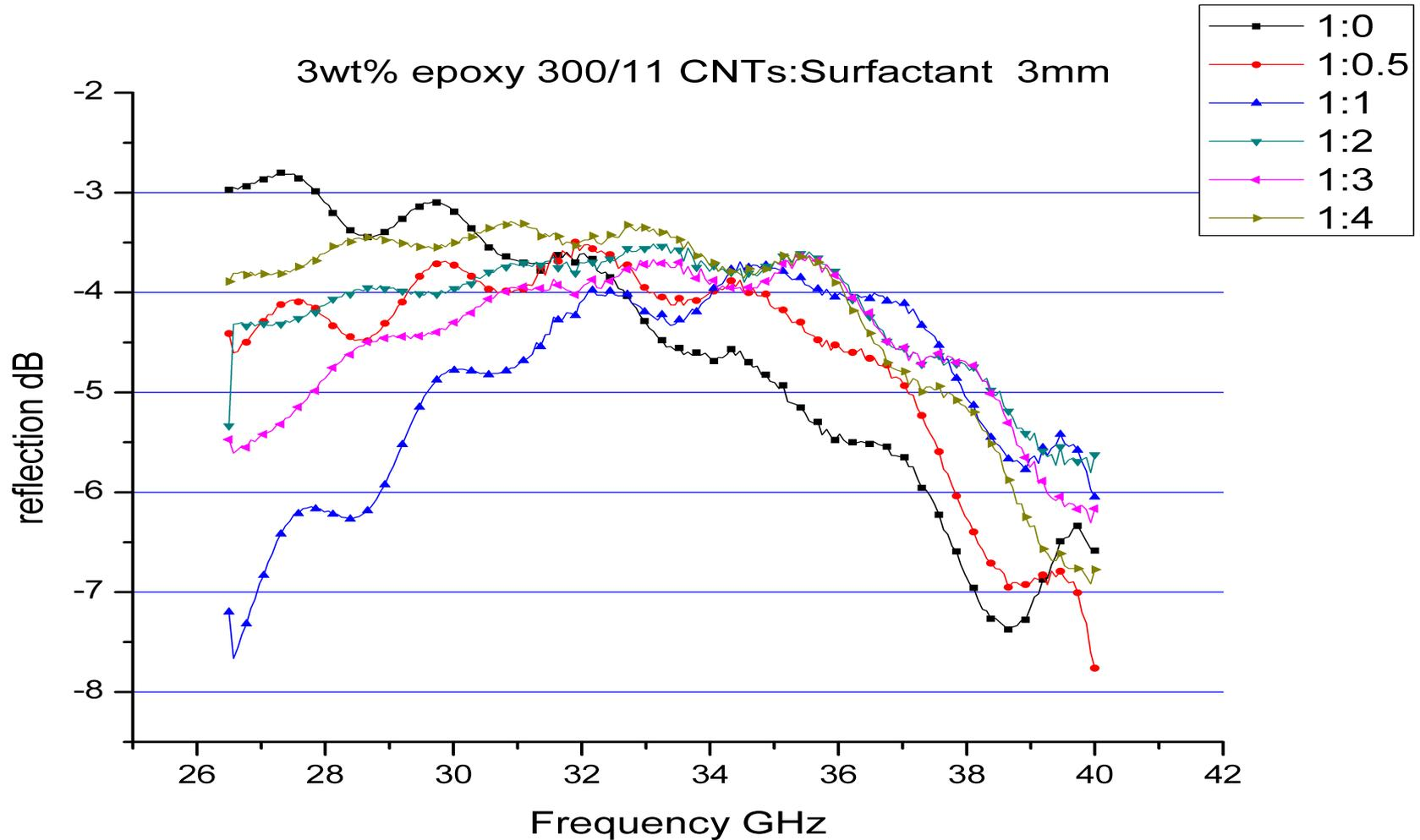
Figure 8 shows that the composites with different ratios of MWCNT/SDBS have different reflection loss properties.
