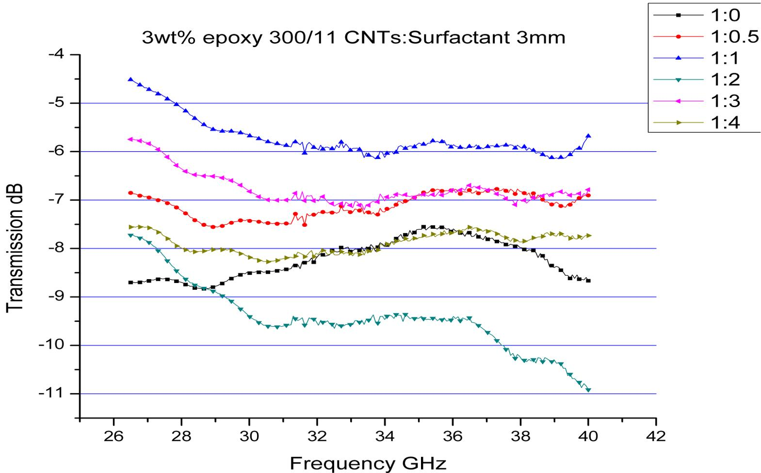
Figure 9 shows that the composites with different ratios of MWCNT/SDBS have different transmission loss properties.
