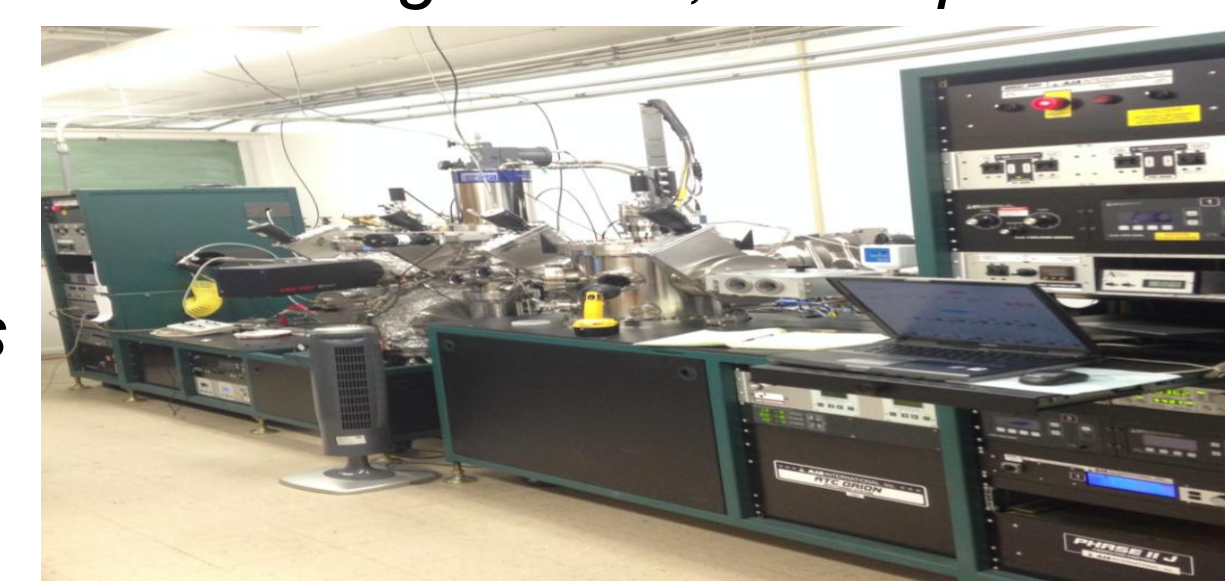
Figure 2. Both the sputtering and electron beam deposition systems in Thin Film lab.
