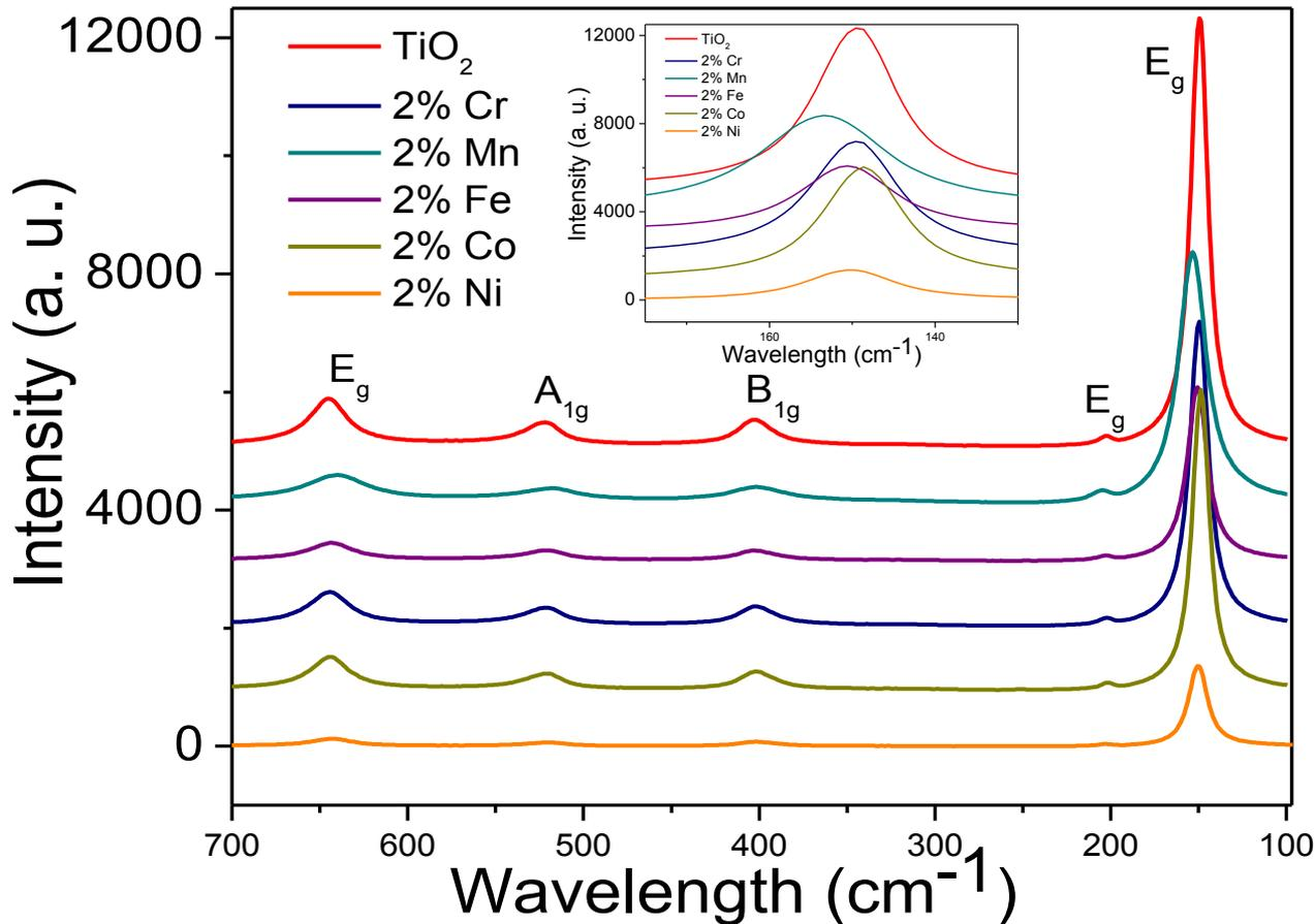
R a m a n spectroscopy data show striking similarities of the spectra of the metal doped powders with that of the undoped sample. This strongly suggests that transition metal ions substitute the Ti<sup>4+</sup> in the host ionic lattice.
