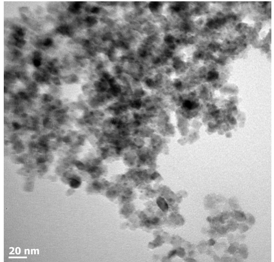
TEM Images of iron-doped TiO<sub>2</sub> nanoparticles
