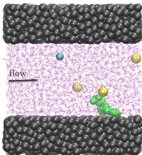
*Side view snapshot depicting the flow of: a nucleotide (green), ions (yellow and blue), and water (purple) through a carbon nanochannel (gray). The nucleotide interacts and adsorbs and desorbs multiple times to the walls as it moves through the channel.*
