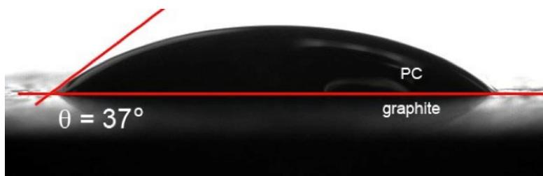
**Figure 1: Propylene carbonate (PC) droplet on graphite.** The low observed contact angle of  $37^\circ$  indicates good wetting behavior, and suggests that PC should effectively fill nanotube forests that are a basis of EDCLs.
