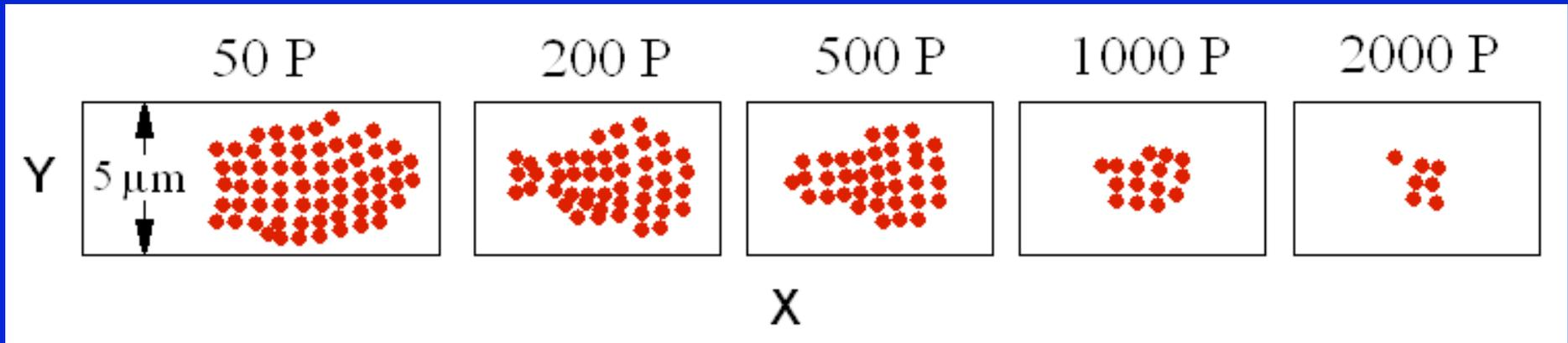
The case of low density of microvilli: 4.0 per  $\mu\text{m}^2$ . The wall shear stress is 0.25 dyn/cm<sup>2</sup>. The P-selectin density is 145 sites/ $\mu\text{m}^2$ ; 5 PSGL-1 molecules per microvillus. The nucleus-to-cytoplasm viscosity ratio is fixed at 2.5. The simulation time is 2.0 s.
