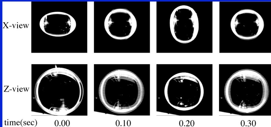
Sequence of 4 video frames depicting a cycle of the normal mode oscillation ( $n=2$ , or quadrupole mode) of a spheroidal sample in an acoustic levitator. Images provided by R. G. Holt (Boston University).
