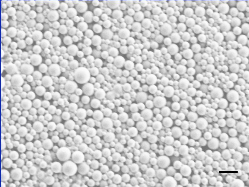
FE-SEM images of PLA microparticles at 3000X. PLA functionalized with mPEG2000-DSPE and b-PEG3350-DSPE. Scale bar is 2  $\mu\text{m}$ . Provided by Joyce Wong (Boston U.)
