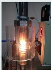
Eddy currents produced within conductors allow volatile powders to be combined while minimizing sample loss
