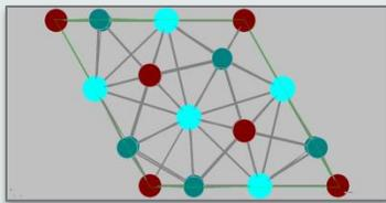
The Fe<sub>2</sub>P crystal structure, a non-centrosymmetric lattice structure, may provide powerful insight into the properties of helimagnets. By synthesizing some of these ternary compounds we hope to produce helimagnetic ordering within materials capable of yielding skyrmions when subjected to a magnetic field
