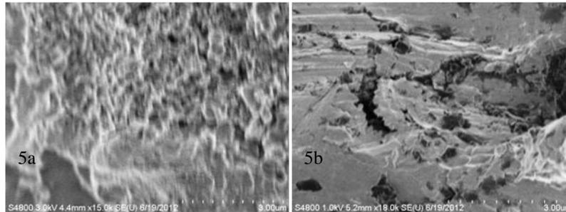
Figure 5: a) SEM image of heater electrode of sample 6, fraction 6 (not blackened) at  $3\mu\text{m}$ . b) SEM image of heater electrode of sample 6, fraction 8 (blackened) at  $3\mu\text{m}$ . The structural changes are easily seen.
