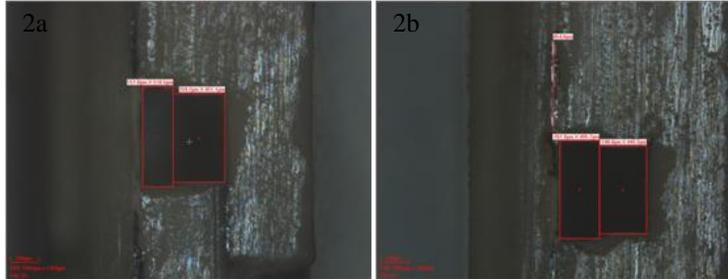
Figure 2 a) and b): Sample 2 (Raw sample), fractions 1 and 8 respectively. There is no noticeable difference in the size of the hole.
