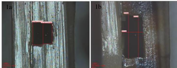
Figure 1 a) and b): Sample 6, fractions 1 and 8 respectively: Noting the difference in hole size as well as color.
