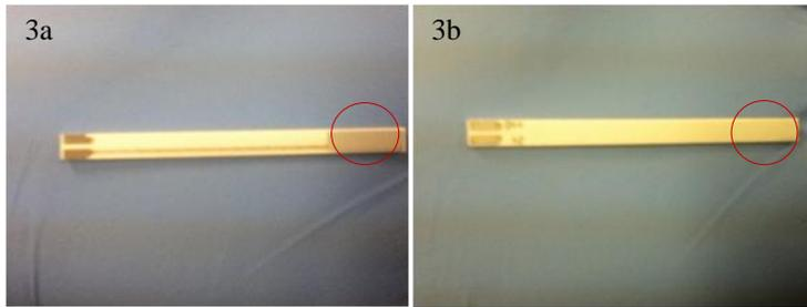
Figure 3 a) Sensor Side and b) Heater Side of a Bosch HEGO sensor. The outlined area is where the blackening occurs (Fraction 8). The opposite end is where the sensor is placed in the housing (Fraction 1).
