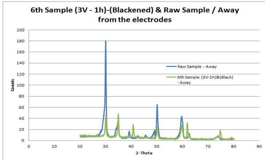
Figure 4: XRD plot comparing the Raw Sample and the Blackened (6th) Sample
