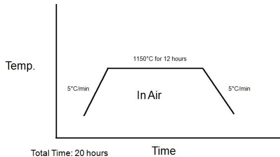
Figure 5 Decarbonization heating profile for high temperature furnace.
