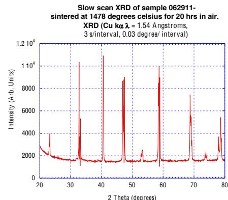
Figure 10 X-ray diffraction pattern for sample #062911 after sintering
