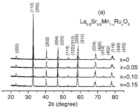
Figure 9 X-ray diffraction pattern of  $\text{La}_{0.5}\text{Sr}_{0.5}\text{Mn}_{1-x}\text{R}_{\text{x}}\text{O}_3$
