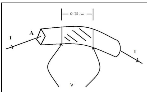
Figure 13 Sketch of four probe method on the sample
