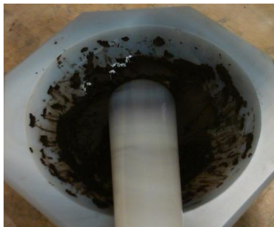
Figure 1 Reactants being mixed together ( 2\text{La}_2\text{O}_3 + 4\text{SrCO}_3 + 8\text{MnO}_2 )
