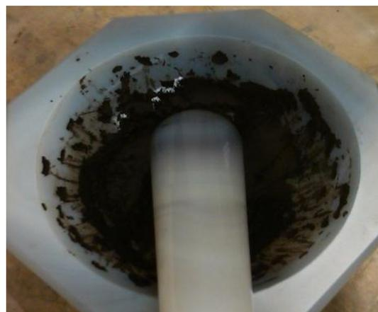
Figure 1 Reactants being mixed together ( $2\text{La}_2\text{O}_3 + 4\text{SrCO}_3 + 8\text{MnO}_2$ )
