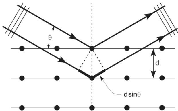
Figure 3 The Scattering of X-Rays from crystal Planes
