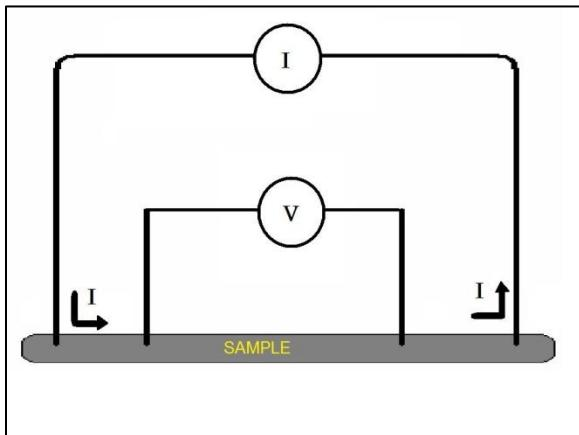
Figure 12 An illustration of the four probe method
