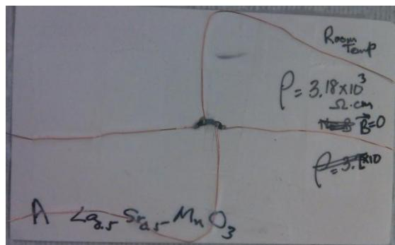
Figure 14 Four leads were attached to the sample with silver paint employing the 4-probe method.
