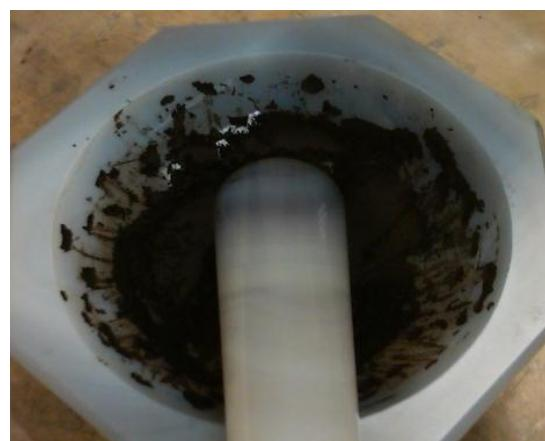
Figure 1 Reactants being mixed together (2La<sub>2</sub>O<sub>3</sub> + 4SrCO<sub>3</sub> + 8MnO<sub>2</sub>)
