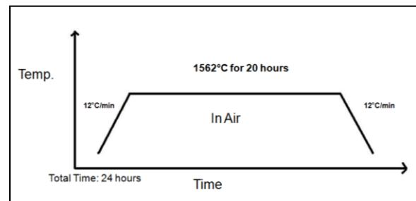
Figure 8 Heating profile for Sintering of sample #062911
