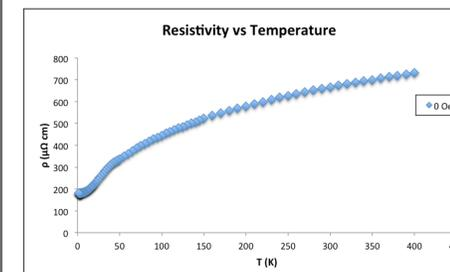
The resistivity data displays a behavior consistent with a that of a metallic material and a phase transition near 40K of unknown character.
