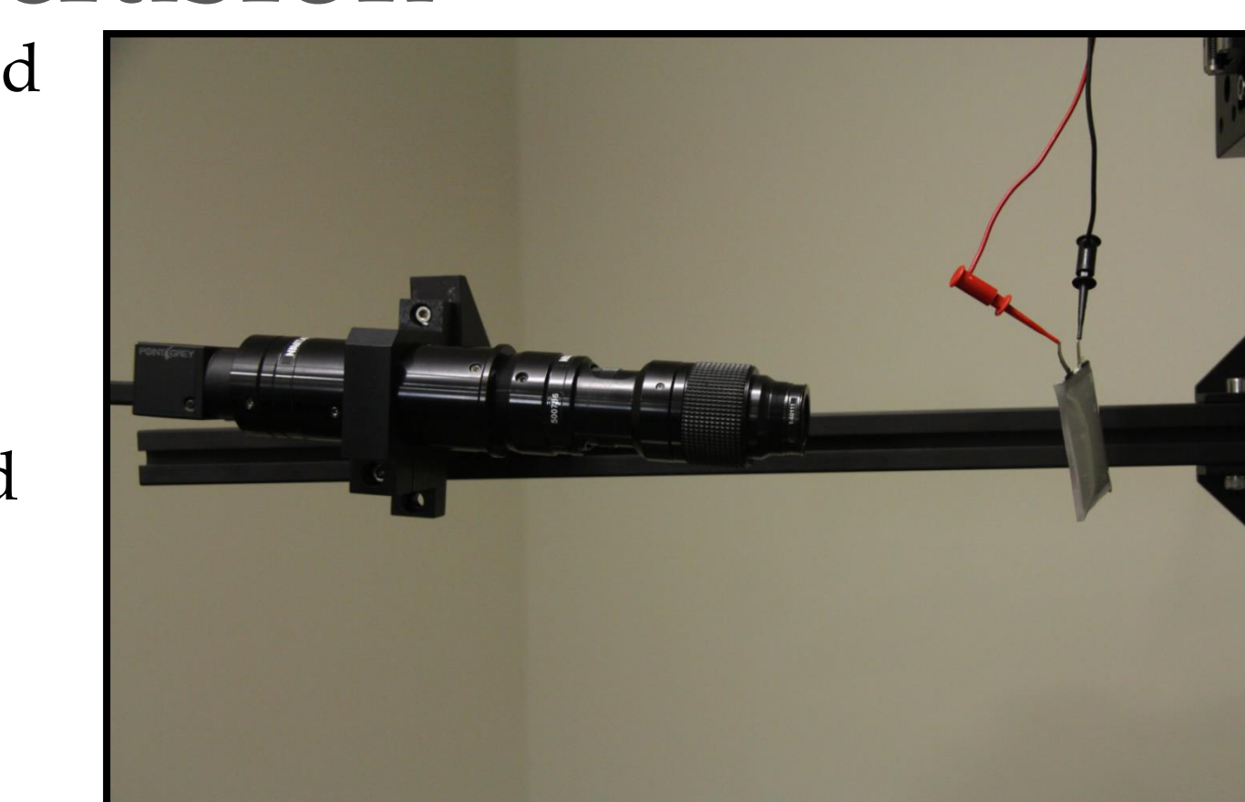
Figure 10: Fully assembled machine with long working distance microscope aimed at battery sample
