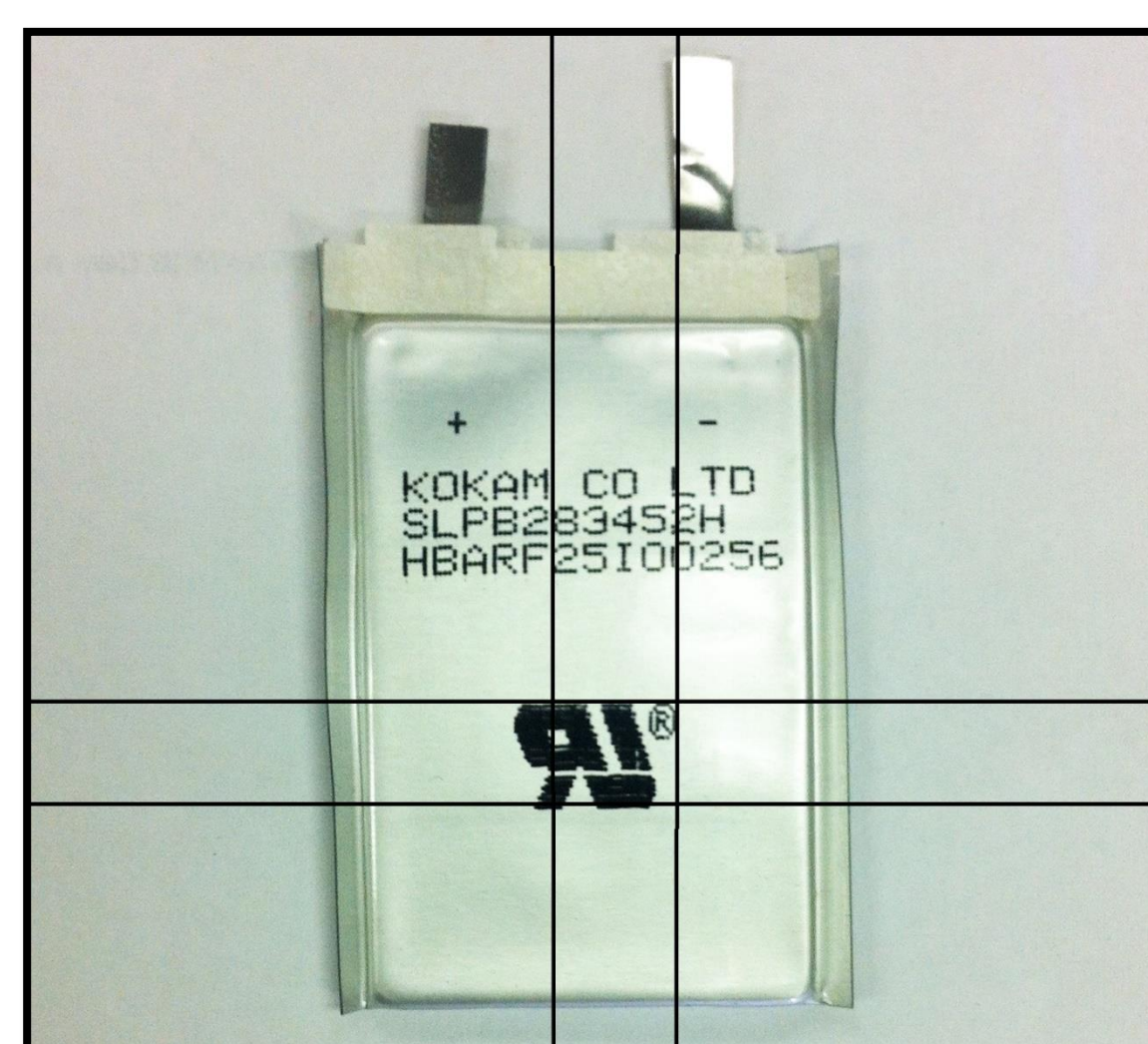
Figure 1: Battery sample with intersecting lines depicting the miniscule 3 mm 2 field of view
