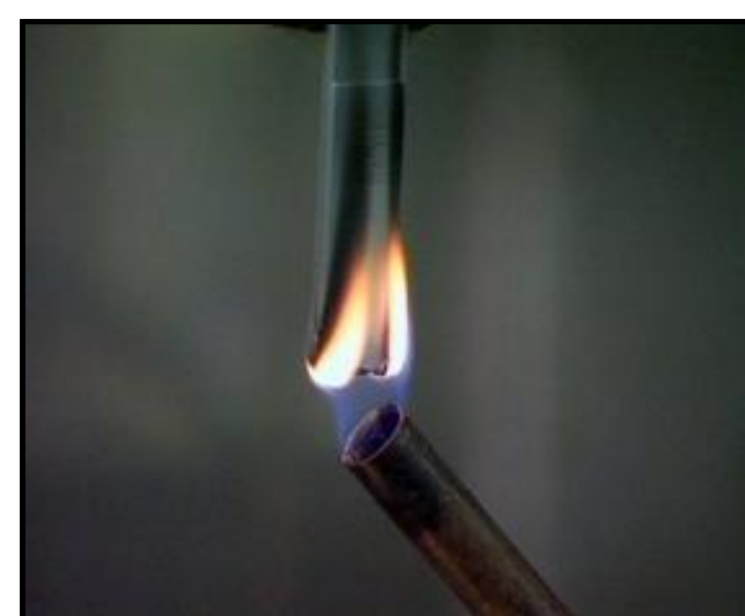
Figure 3: Flame retardant sample beginning to warp under heat
