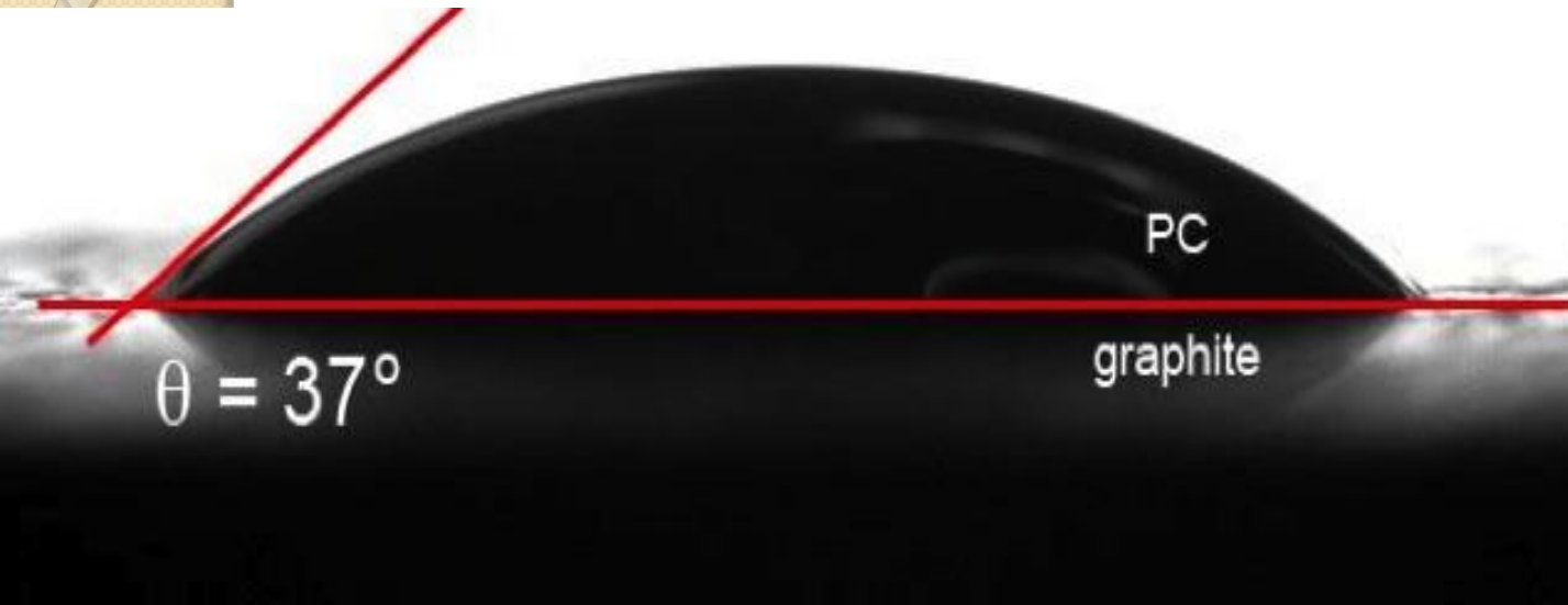
FIG. 3. <Top> Contact angle of a propylene carbonate droplet on a graphite surface. [4]
