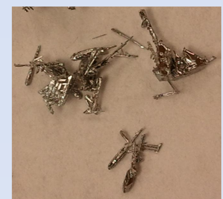
Clusters of needle shaped single crystals of MnSi
