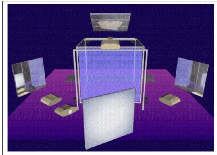
**Figure 1. Schematic [4] of the CAVE at Southern's College of Engineering. Projection is via mirrors used to set the correct optical distance equal to the projector's throw.**
