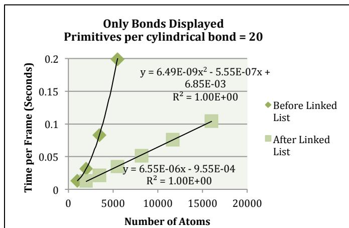
**Figure 5. Variation in the execution time of the modified and original codes for the display of bonds alone. The quadratic dependence of the execution time of the original code on the number of atoms is changed to a linear one via the use of linked lists in the modified code.**
