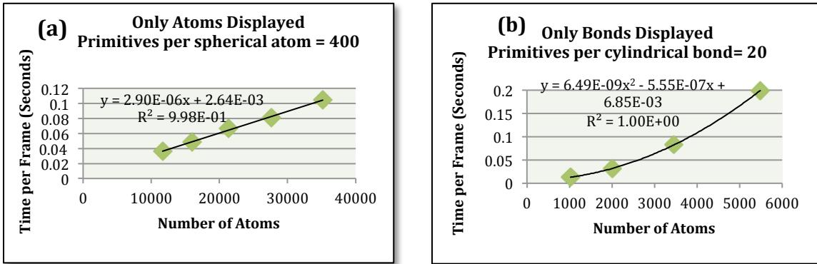
**Figure 2.** Variation in the execution time of the original code on the  $2 \times$  dual core, 3.22 GHz, Opteron when visualizing a BCC lattice with all 8-bonded atoms. (a) Only atoms displayed as spheres. (b) Only bonds displayed as cylinders.
