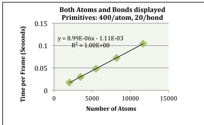
**Figure 6. Variation in the execution time of the modified code to display both atoms and bonds. The linear dependence of this execution time on the number of atoms follows from the same dependence when displaying atoms alone (Fig. 2a) or bonds alone (Fig. 5).**
