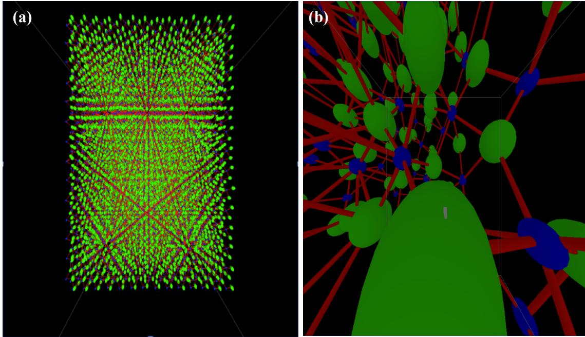
**Figure 7. Application of the code to an Alumina system. (a)** shows a full view with ~47,000 atoms. Blue spheres represent Aluminum, green spheres represent Oxygen, and bonds are in red. **(b)** shows a close-up view of the system. The structure is complex with 6-bonded Aluminum atoms and 4-bonded Oxygen atoms.
