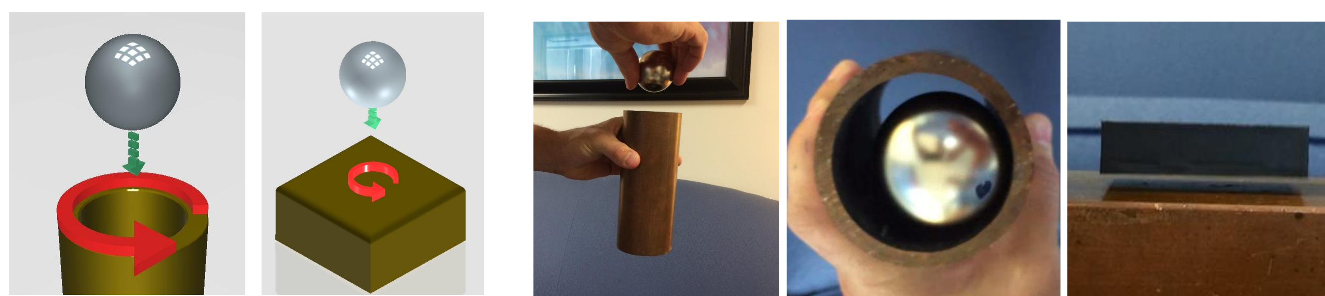
Illustrations created in Autodesk Inventor to show the current being created as the magnet falls.
