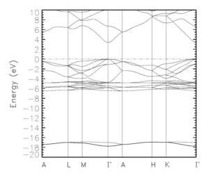
Calculated electonic energy bands of zinc oxide (ZnO). The direct band gap at the gamma point is 3.4 eV.
