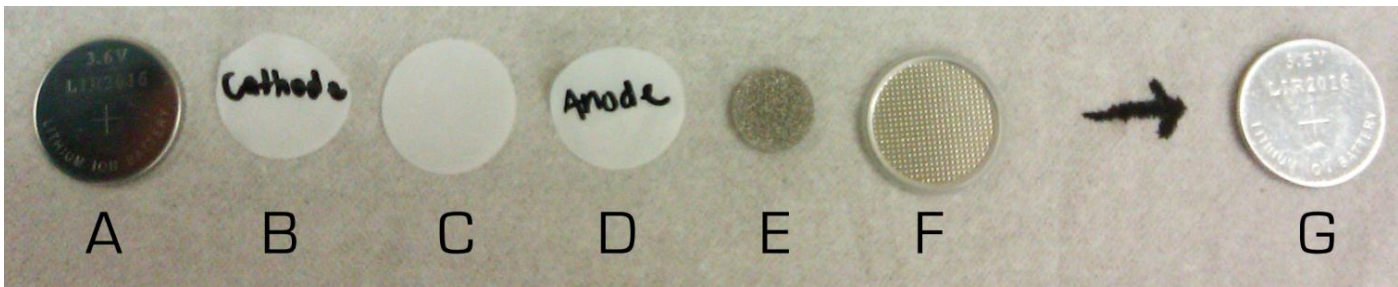
Assembly of a lithium ion coin cell. (A) positive terminal; (B) cathode; (C) insulator; (D) anode (lithium); (E) current collector (nickel foam); (F) negative terminal; (G) completed lithium ion coin cell
