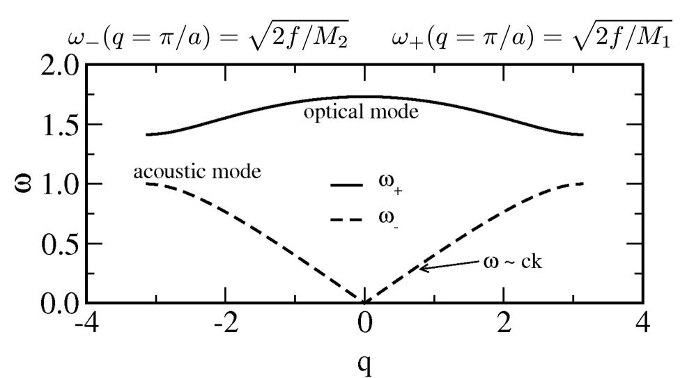
Looking at the optical mode at q = 0,  $\omega_{+}(0) = 2f/\mu$
