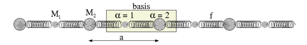
Consider a linear chain of oscillators composed of a twoelement basis with different masses, M<sub>1</sub> and M<sub>2</sub> and equal strength springs with spring constant f. It has the potential energy
