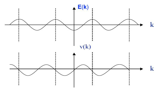
In a DC electric field (constant), electrons reverse its motion direction (v changes sign) at the B-zone boundary
