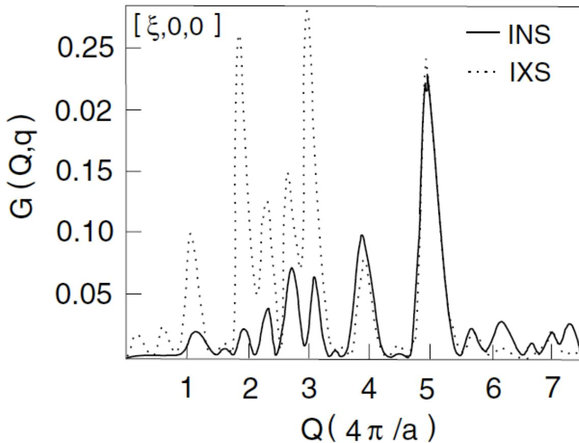
**Figure 13.** The structure factor ( $G(Q, q)$ ) of  $\alpha\text{-SiO}_2$  for the longitudinal acoustic mode along  $[\xi, 0, 0]$  for x-rays (broken line) and neutrons (full line) calculated by Halcoussis (1997).
