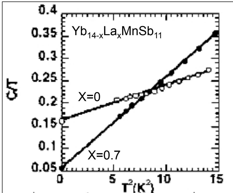
$$C_{total} = C_{electron} + C_{phonon} = \gamma T + \beta T^3$$
