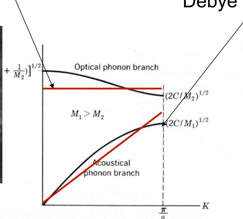
**Figure 7** Optical and acoustical branches of the dispersion relation for a diatomic linear lattice, showing the limiting frequencies at  $K = 0$  and  $K = K_{\max} = \pi/a$ . The lattice constant is  $a$ .
